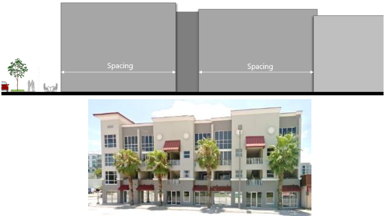
Figure 5 - 12: Example of Building and Roof Articulation
