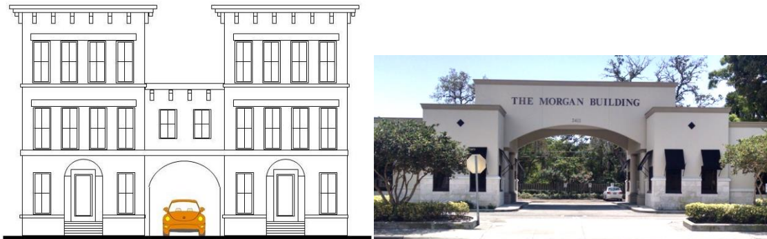
Gateway feature designed to meet minimum building frontage. Notes: Not to scale. Floor above the gateway is not required.
