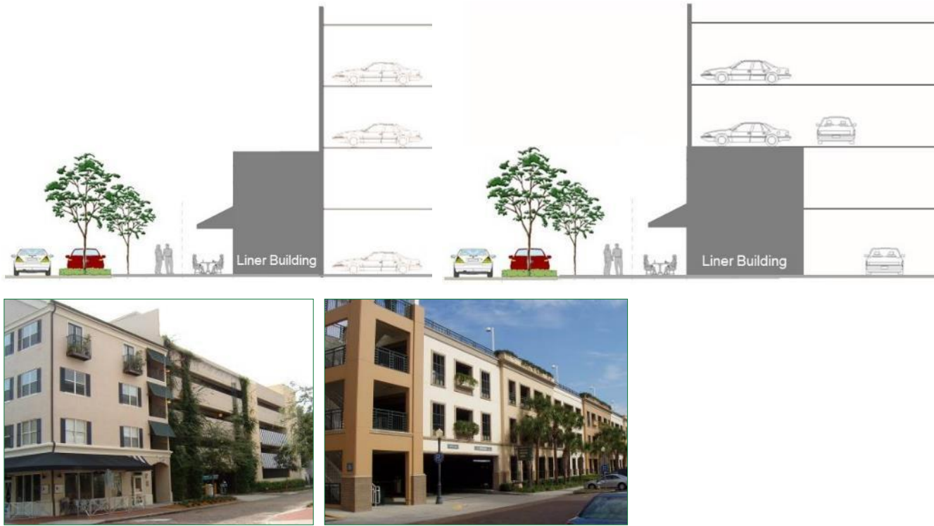
Figure 5 - 43: Parking Garages and Liner Buildings
